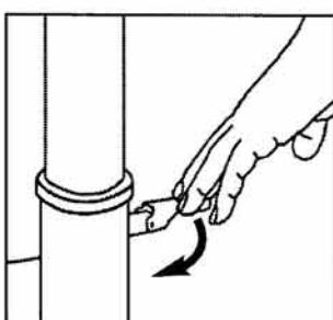
4 Flip the lock handle down to activate the lock.
