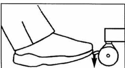
Step down on the tab at the front of the wheel.
