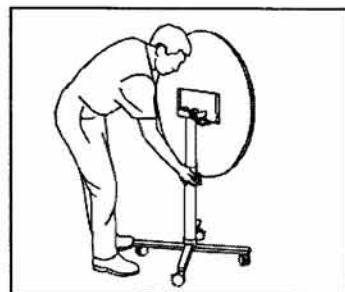
1 Locate the column lock at the center of the column.
