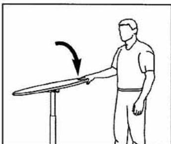
Grasp the table top and carefully rotate down until it is locked in place.
