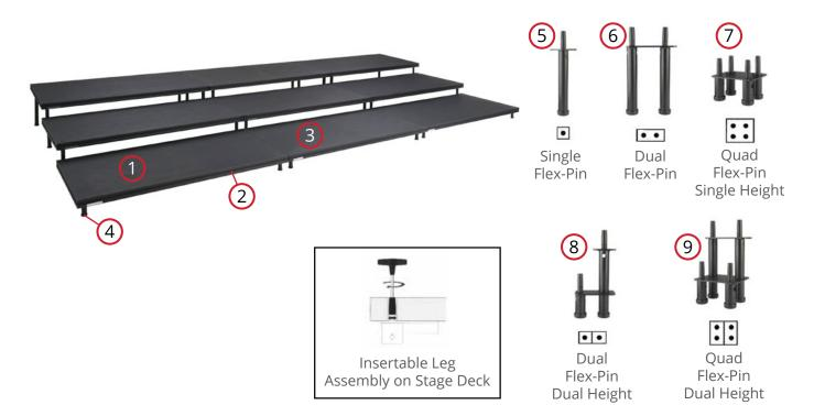
The structural decks are constructed with a honey-comb core sandwiched between 3/8" thick plyboards. Deck is light-weight, very strong and quiet, with strength to support 125lbs. per square foot (610 kg. per square meter), which meets or exceeds most building requirements.
