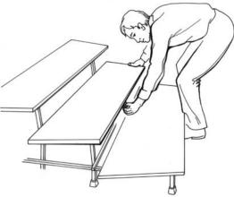
3. Move additional units into place, unfold, reverse steps if necessary, and align.
