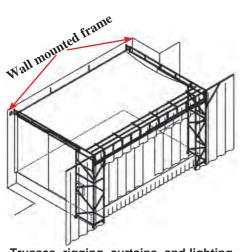
**Trusses, rigging, curtains, and lighting** are supported by wall mounted frames. Designed with security in mind: The corner towers are connected to front and folding top trusses that lock into place. Locks release from ground level.
